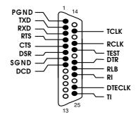
Figure 6. V.24 DCE Interface
